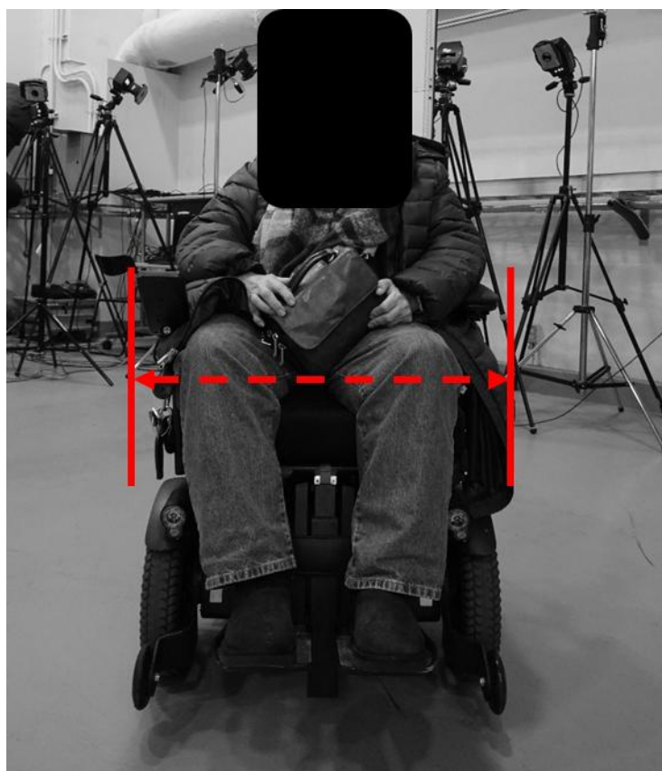
Figure 2. Front-view image of a power wheelchair. The red, dashed arrows depict an example of the occupied measurement (e.g. from widest points on the person or device, with consideration of personal items and accessories)
