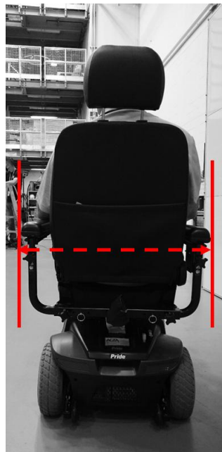
Figure B-1. Rear-view image of a scooter. The red, dashed arrows depict an example of the unoccupied measurement (e.g. from arm rest to arm rest, without considering the person)
