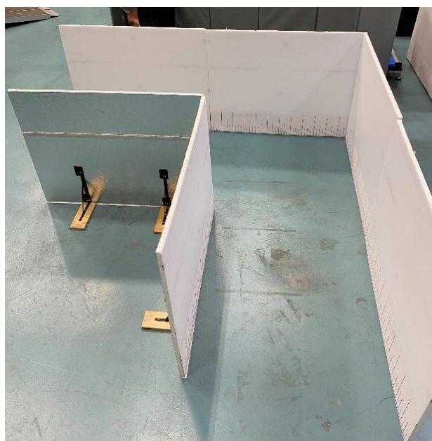
Figure 11. Image of corridor with a 90-degree turn, bounded by foam walls. The walls are movable, allowing the space to progressively reduce in size.
