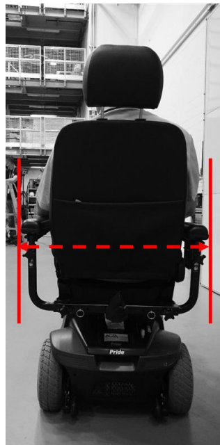
Figure A-1. Rear-view image of a scooter. The red, dashed arrows depict an example of the unoccupied measurement (e.g. from arm rest to arm rest, without considering the person)
