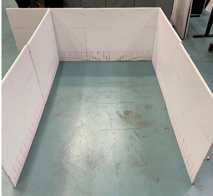
Figure 7. Image of square space bounded by foam walls, used for continuous and non-continuous turning area. The walls are movable, allowing the space to progressively reduce in size
