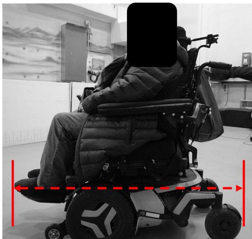
Figure 3. Side-view image of a power wheelchair. The red, dashed arrows depict an example of the occupied measurement (e.g. from front-most to rear-most point of the person or device, with consideration of personal items and accessories)
