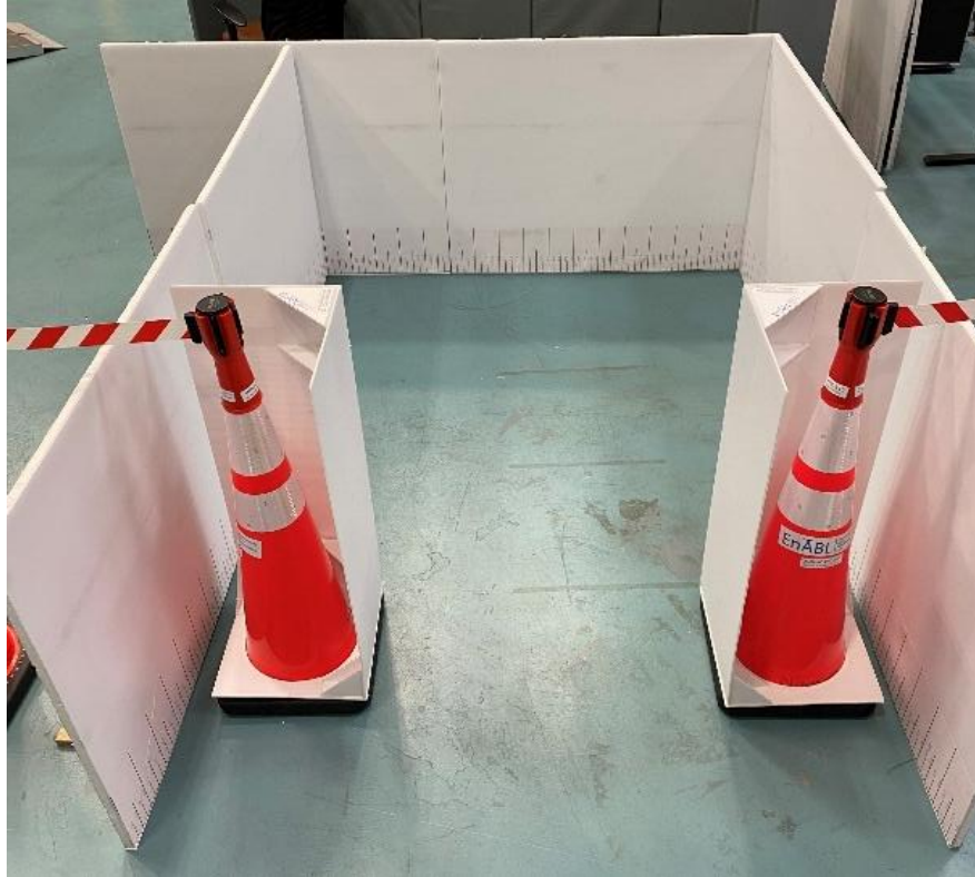
Figure 9. Image of square space bounded by foam walls. A middle entry/exit door is shown in the image, created using two pylons. The walls are movable, allowing the space to progressively reduce in size. The door width remained fixed at 850 mm.
