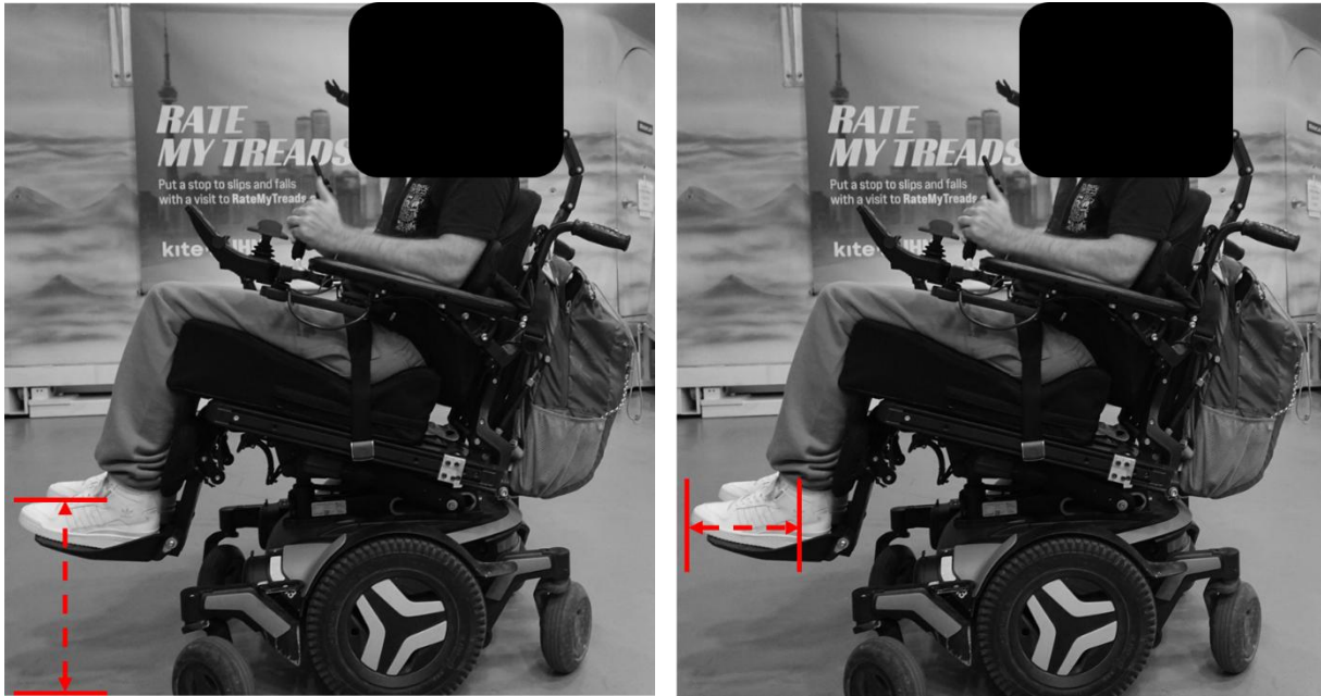
Figure 6. Side-view image of a power wheelchair. The red, dashed arrows depict an example of toe height (left) and toe depth (right).
