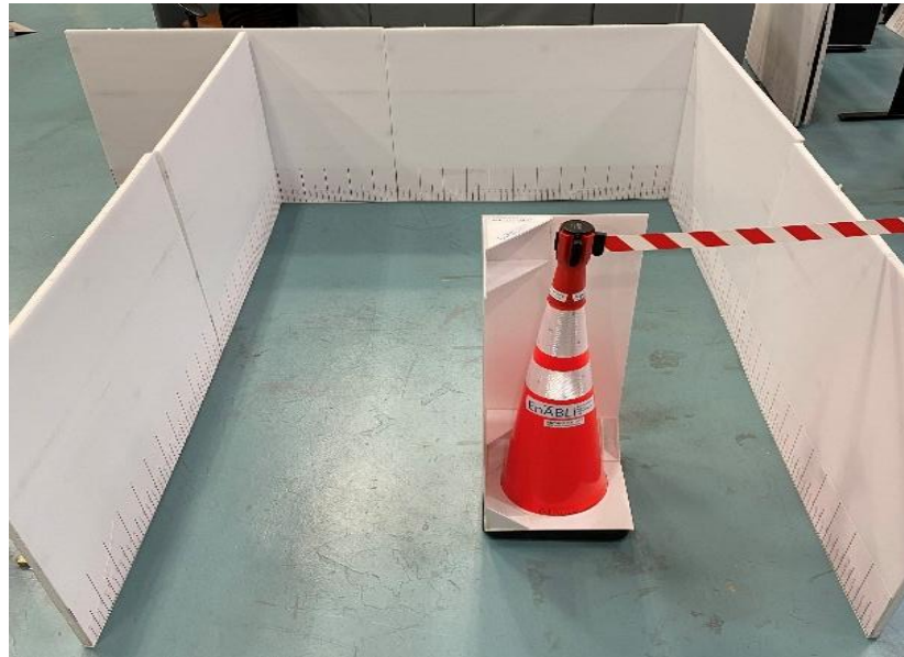
Figure 8. Image of square space bounded by foam walls. A left-corner entry/exit door is shown in the image, created using a pylon. The walls are movable, allowing the space to progressively reduce in size. The door width remained fixed at 850 mm.
