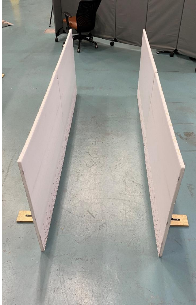
Figure 10. Image of straight corridor, bounded by foam walls. The walls are movable, allowing the corridor width to progressively reduce in size.
